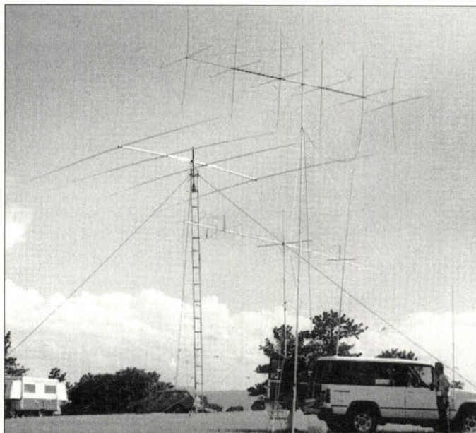
Fig. 1: A general view of some of the Field Day antennas at NOAUS, showing a 50MHz 6-element quad, a 4-element mono-bander for 14MHz and a 22-element array for 144MHz.
